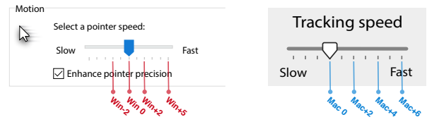
Figure 1: Operational system settings compared in the study. MS Windows 10 v. 1909 (left) and OS X 10.6.7 (right) available acceleration settings on each system's mouse speed slider.
